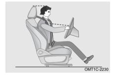
The shoulder belt should be over the shoulder center and close to the chest, kept away from the neck, the lap belt should be closed to the hips but not stomach.
