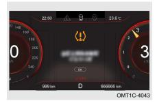
When vehicle speed is more than 30 km/h, if the tire pressure monitoring system has not received the radio-frequency signal from one or more sensors for 10 minutes, TPMS will send system malfunction alarm,
