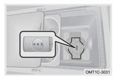
When smart key battery is low or signal is seriously interfered, engine start stop function will not work normally. In this case, start engine according to following steps:
