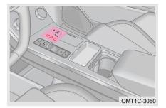
After driver shifts the shift lever to D, vehicle upshifts and downshifts automatically according to speed without manual intervention.
