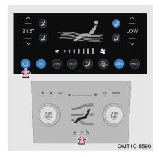
The air conditioning system can be turned off by operating A/C switch button on air conditioning control panel or soft button on the display screen.
