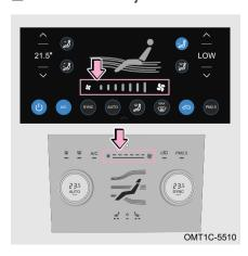
The airflow volume can be adjusted by operating the airflow volume adjustment button on air conditioning control panel or the soft button on display screen.
