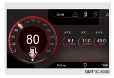
Fuel gauge is used to indicate current amount of remaining fuel in the fuel tank.
