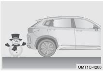
Radar sensors cannot detect objects that easily absorb ultrasonic waves such as soft snow, cotton, sponge, etc.
