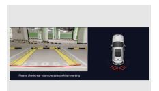
When a radar sensor detects an obstacle, audio head unit displays corresponding distance information and speaker sounds.
