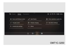
On vehicle setting screen, door and window control, seat position, exterior light setting, driving assist system setting, wireless charging, back door control, outside rear view mirror setting and other relative functions can be set.
