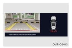
Move electronic shift switch to R to enter reversing view monitor screen, and reversing view monitor screen will display the reversing view monitor and lane guideline.
