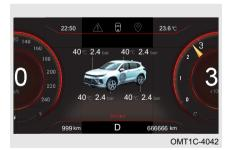
When ENGINE START STOP switch is turned to ON mode, on driving information screen, push down steering wheel combination button " to switch to tire pressure display screen.
