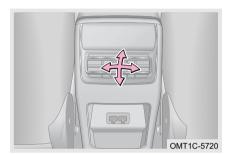
Move outlet adjustment lever up, down, left or right by hand to adjust direction of airflow.
