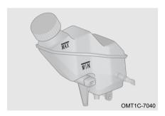
Brake fluid level should be between the "MIN" and "MAX" marks. If the level is in the "MIN" mark or below, add brake fluid and contact EXEED authorized service station for inspection and repair immediately.
