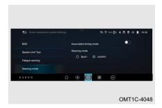
Electric power steering system is equipped with two modes (SPORT/COMFORT). The default steering mode of electric power steering system (EPS) is comfort mode when the vehicle first works.
