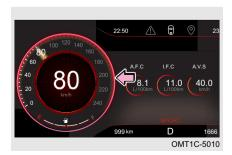
Speedometer uses digital to indicate current vehicle speed. (Unit: km/h).
