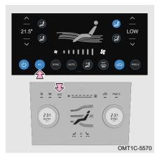
The air conditioning cooling can be achieved by operating A/C switch on air conditioning control panel or soft button on display screen.
