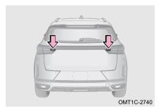
Turn ENGINE START STOP switch to ON mode, shift the shift lever to R, back-up lights come on.
