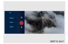
The driving recorder is connected to the audio head unit through Wi-Fi and is displayed and operated on the audio head unit. Click driving recorder application to enter the real-time screen of it. Click the upper left corner to return to the audio main screen and exit the driving recorder screen.
