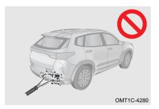
High pressure water flow such as water guns or excessive external forces may cause damage to the radar sensors. Do not pinch or impact the radar sensor, or it may cause abnormal operation.
