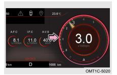
Tachometer uses digital to indicate current engine speed (Unit: x1000 rpm).
