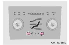
After vehicle is started and seat is in stationary, the seat heater switch is at 2-level heating (2 indicators on) as pressing first time. Press it again to enable 1-level heating (1 indicator on). Press it at third time to turn off the function.
