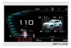
Remind that front seat belt is not buckled or fastened firmly:
