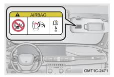
This sticker is attached to front passenger sun visor and used to remind you that the vehicle is equipped with front airbag (SRS). Observe the following precautions:
