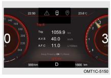
It can be used to calculate distance between two locations after Trip A / Trip B is reset.
