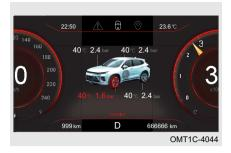
When tire inflation pressure is less than 1.75 bar, and vehicle continues to drive at a speed higher than 30 km/h, system will send low pressure warning within 5 minutes.
