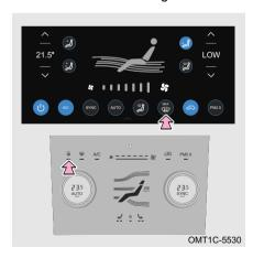
The defog/defrost function can be achieved by operating front windshield defog and defrost button on air conditioning control panel or the soft button on display screen.
