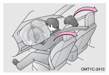
Seat belt pretensioner is designed to assist front airbag in the event of a severe impact.
