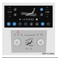
After starting the vehicle, press the rear defrosting button. If the indicator comes on, it indicates that the rear defrosting/outside rear view mirror heater defrosting function starts to work. If the indicator goes off, it indicates that the rear defrosting/outside rear view mirror heater defrosting function stops working.
