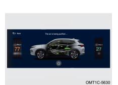
Operate PM2.5 button on air conditioning control panel or soft button on display screen to enable the one-button purification function of air conditioning system to purify the air inside the vehicle.
