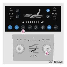
The single/dual mode can be switched by operating the single mode button on air conditioning control panel or the soft button on display screen.
