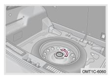
Open back door, lift the luggage compartment carpet and take out the storage box and tool bag. Rotate fixing bolt of spare tire counterclockwise to remove it, and then take out the spare tire.
