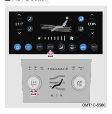
The air conditioning AUTO mode can be turned on by operating AUTO button on air conditioning control panel or soft button on the display screen.
