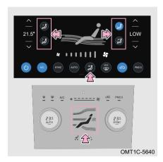
The adiustment mode can be achieved by touchina mode adjustment area (window blowing mode, face mode and foot mode can combined to use) conditioning control panel or the soft button on display screen
