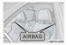
When vehicle is subjected to side collision and deployment conditions are met, seat airbag of impacted side deploys. Besides seat belt, front seat side airbag is a kind of device that can provide more protection for driver and front passenger.
