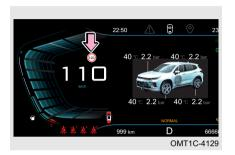
Speed limit assist system alarm display:
