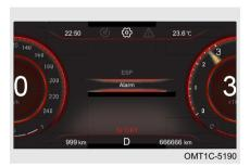
Overspeed alarm can be set by operating steering wheel combination buttons:
