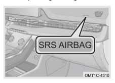
When front passenger airbag is triggered, the airbag cover will be opened from instrument panel and the airbag deploys.
