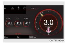
When ENGINE START STOP switch is turned to ON mode, it indicates current engine coolant temperature.
