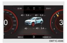
When the tire pressure is more than 3.5 bar, the tire pressure value will display –, but the temperature value will be displayed normally; When the tire pressure is less than 3.5 bar, the normal display will be restored within 5 minutes.
