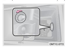
Turn it counterclockwise to open outlets, and turn it clockwise to close outlets.
