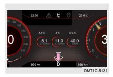
Display the currently selected gear range information (in manual mode or current gear range).
