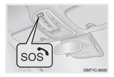
ERA-GLONASS ic а kind of emergency call function. When vehicle is involved in a certain level of impact (airbag inflated) or when driver or passenger is in emergency and rescue is required, emergency information can be sent to service center by operating button manually, then the center will track vehicle location and promptly offer received rescue according to information.
