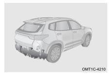
When radar sensor surfaces are frozen, they will not detect any obstacle.
