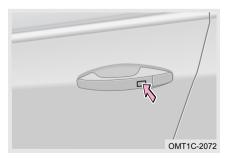
Carry smart key and touch the sensor on door handle. After door handle sensor recognizes locking signal, the turn signal indicator will flashes once and the door will automatically lock.
