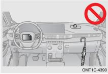
Do not attach anything to or lean anything against the areas such as the instrument panel, steering wheel and lower portion of the instrument panel. These items can become projectiles when driver airbag or front passenger airbag deploys.
