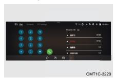
In Setting - System setting --Connection - Bluetooth phone, connect phone Bluetooth to audio first, then click phone in main screen to enter Bluetooth phone screen.
