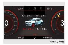
When tire temperature of vehicle is higher than 85° C, and vehicle continues to drive at a speed higher than 30 km/h, system will send high pressure warning within 5 minutes.
