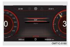
ESP function can be set by operating steering wheel combination buttons:
