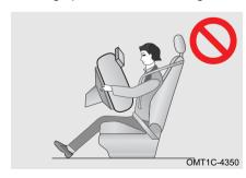
Always keep airbag inflation path clear. It is forbidden to place anything (mobile phone, etc.) between the occupant and the airbag. It is forbidden to fix or place any object on or near the airbag cover. If there is an object between occupant and airbag, the airbag may not deploy according to design path, or the airbag may push object to occupant's body, causing serious injury or even death.
