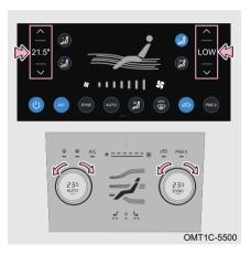
The A/C temperature can be adjusted by operating the driver side temperature adjustment knob/front passenger side temperature adjustment knob on air conditioning control panel or the soft button on display screen.
