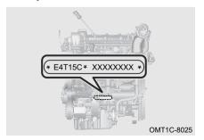
Engine number is located on engine block as shown in the illustration.
