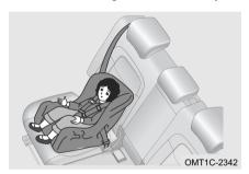
The forward-facing child restraint system should be installed facing vehicle traveling direction. It is recommended for group I: 9 - 18 kg.
