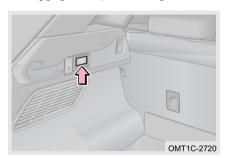
When back door is opened, luggage compartment light will turn on automatically. When back door is closed, luggage compartment light will turn off immediately.
