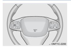
To sound the horn, press area near horn mark on the steering wheel.
