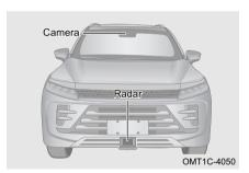
ACC, AEB and FCW share a radar and a camera sensor (If equipped).
