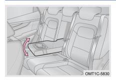
Rear seat is equipped with a folddown armrest with cup holders, fold down the armrest for use.
