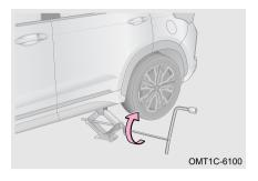
When jacking up vehicle, fit jack rocker into jack and wheel bolt wrench into jack rocker, and turn the wheel bolt wrench clockwise. When the jack touches the vehicle and begins to jack, check if its jacking-up position is proper again.
