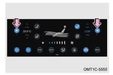
After vehicle is started, the seat ventilation switch is at 2-level ventilation (2 indicators on) as pressing first time. Press it again to enable 1-level ventilation (1 indicator on). Press it at third time to turn off the function.
