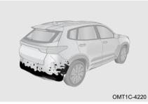
When radar sensors are covered by dirt, snow or mud, they may not detect obstacles.
