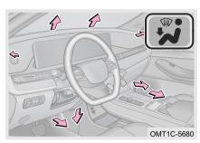
Air flows mainly from floor outlets, front windshield defrosting outlets and side defrosting outlets.
